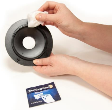
10.5 Wipe the filter adapter clean. Check that the sealing ridge for the particle filter is undamaged.
