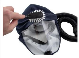
**6.2** If the equipment is more heavily fouled, use a soft brush or sponge moistened with a solution of water and dishwashing detergent or the like. Rinse the equipment and leave it to dry.
