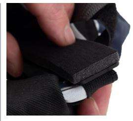
**5.3** Fit the new sweatband. The forehead strap and the sweatband should be mounted edge to edge.
