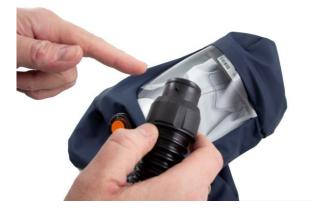
**1.2** Check that the O-ring of the hose is in place.
