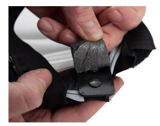
**5.1** Pick away one end of the sweatband so that it is removed together with the tape.
