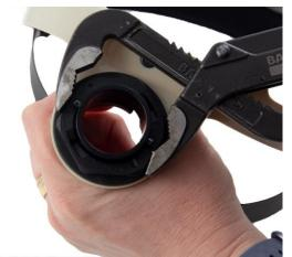
**7.3** Turn the locknut a quarter of a turn to remove it. Use polygrip pliers if the locknut is stiff to turn.
