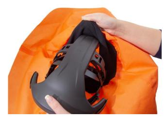
**10.1** Remove the hood from the air-duct by releasing the two fixing grooves and pull off the hood from the head harness and air-duct. Assemble the new air-duct in reverse order or see the instructions in section 1. Assemble.
